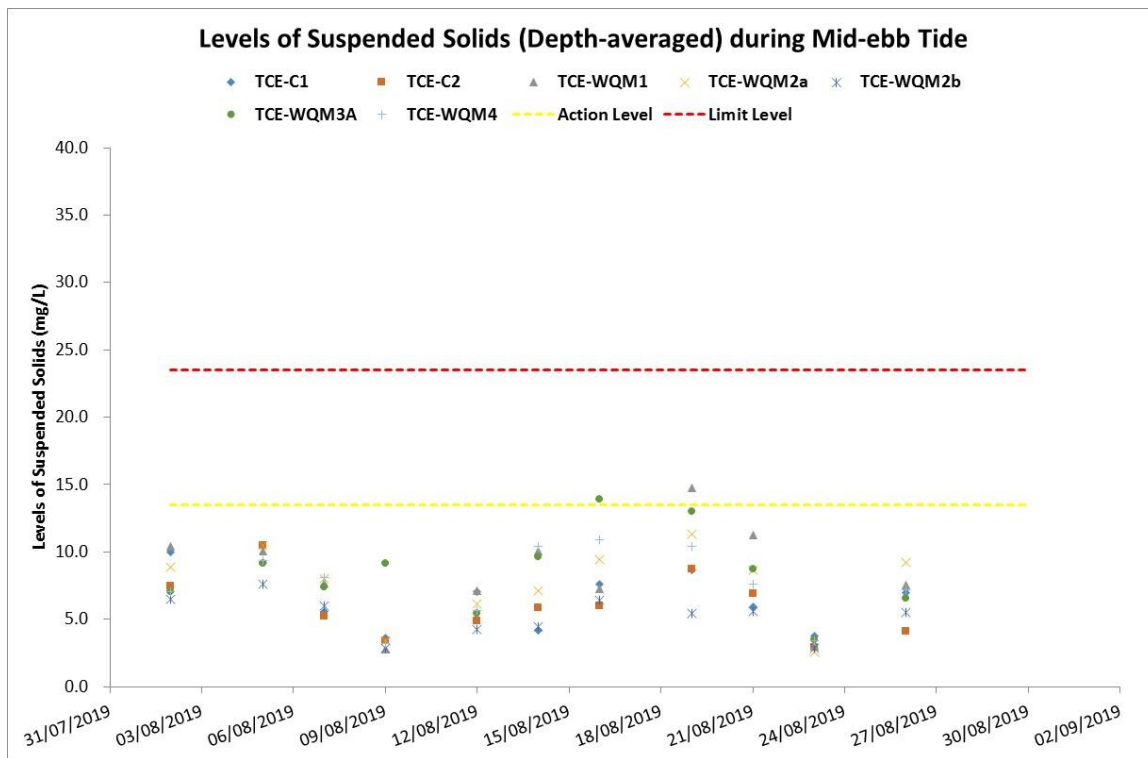
Figure 7: Levels of Suspended Solids (Depth-averaged) (mg/L) recorded at Mid-ebb Tide during the Water Quality Monitoring between 1 and 31 August 2019
