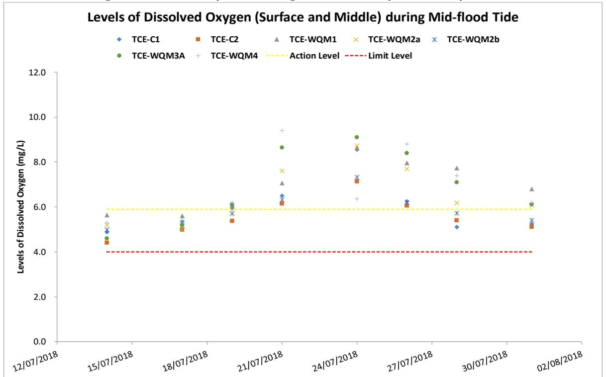
Figure 2: Levels of Dissolved Oxygen (Surface and Middle) (mg/L) recorded at Mid-flood Tide during the Water Quality Monitoring between 13 July and 31 July 2018
